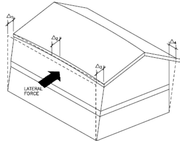
NOTE: IF STIFFNESS OR LOAD IS NONSYMMETRICAL, BUILDING ROTATION OCCURS ( $\Delta_1 \neq \Delta_3$ ) AND LOADS ARE DISTRIBUTED BY TORSION ( $\Delta_4 \neq 0$ ) AS WELL AS BY DIRECT SHEAR IN THE DIRECTION OF THE LATERAL FORCE. THIS CONDITION VARIES BUT IS A REALITY FOR MOST DESIGNS.  $\Delta_2$  IS THE BENDING DEFORMATION OF THE HORIZONTAL DIAPHRAGM (I.E., ROOF).
