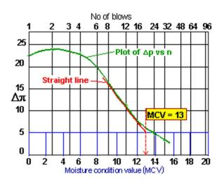
After plotting  $\Delta \pi$  against the number of blows n, a line is drawn through the steepest part.
