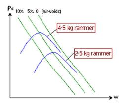
Laboratory compaction tests
