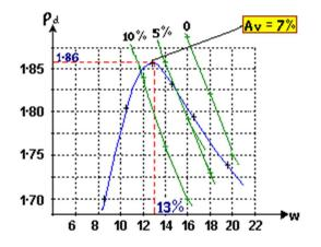
The **optimum air-voids content** is the value corresponding to the maximum dry density  $(1.86 \text{ Mg/m}^3)$  and optimum water content (12.9%).
