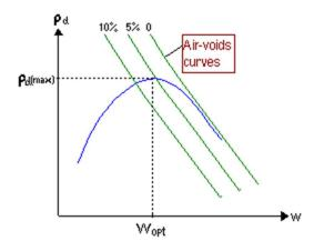
The maximum dry density is controlled by both the water content and the air-voids content. Curves for different air-voids contents can be added to the  $\rho_d$  / w plot using this expression:
