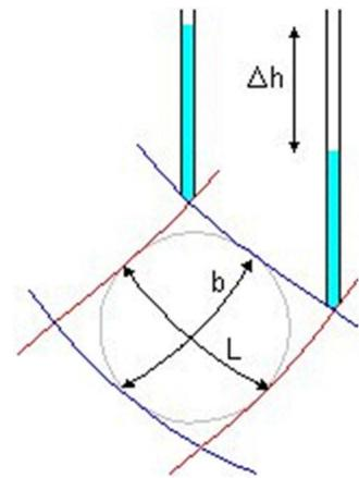
There is an advantage in displaying or sketching flownets in the form of curvilinear 'squares' so that a circle can be inscribed within each four-sided figure bounded by two equipotentials and two flow lines. Then  $b = L$  and  $q = k\Delta h$  so the flow rate through the flow channel is the permeability multiplied by the uniform interval  $\Delta h$  between equipotentials.
