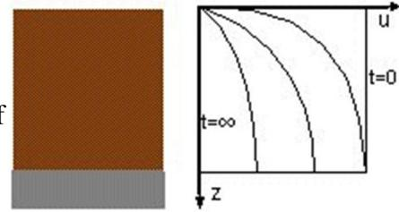
The time-dependent transient change in pore pressure that occurs as a result of some perturbation, and associated change in effective stress is called **consolidation**.
