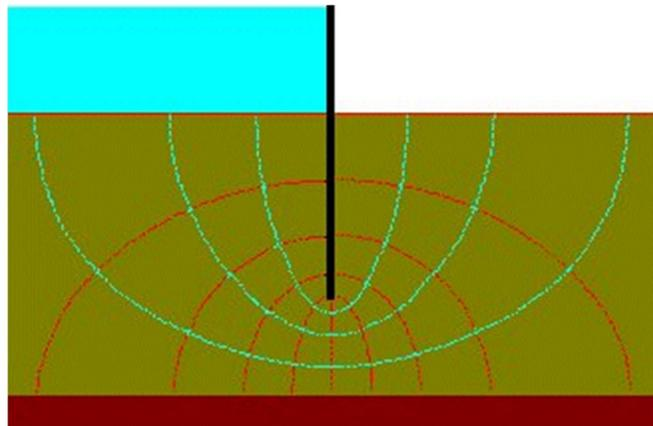
**flow lines** indicating the direction of seepage down a hydraulic gradient
