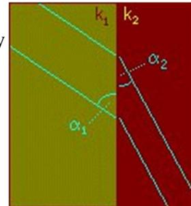
It is not possible to construct a flow net with curvilinear squares on both sides of the interface unless the head drop between equipotentials is changed in inverse proportion to the permeability ratio.
