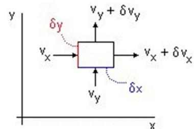
For a rectangular element with dimensions  $\delta_x$ ,  $\delta_y$  and unit thickness, in the  $x$  direction the velocity of flow into the element is
