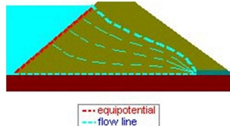
Total head changes and elevation changes thus match and for equal head intervals  $\Delta h$  between equipotentials there must be equal vertical intervals between the points of intersection of equipotentials with the phreatic surface.
