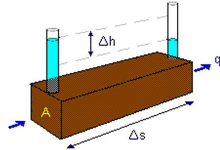
The coefficient of permeability of a soil is a measure of the conductance (i.e. the reciprocal of the resistance) that it provides to the flow of water through its pores.
