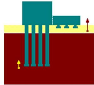
Although older buildings are unlikely to be damaged, modern structural forms, such as those in the diagram, would be vulnerable. If water levels rise causing the clay to swell, the two parts of the building with differing foundation levels will heave by amounts which could differ by up to 100mm.
