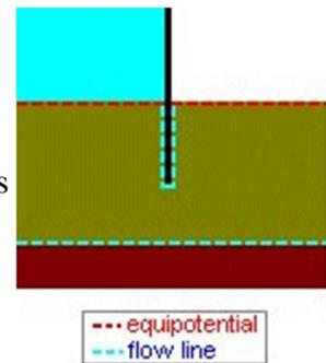
For the situation shown, with flow occurring under a sheet pile wall, the
