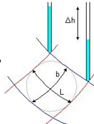
These pore water pressures are partly supporting the weight  $\gamma_w bL$  of water in the element and partly providing the seepage force. It is found that the seepage force is
