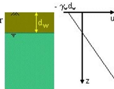
Where the water table is deeper, or where evaporation is taking place from the surface, saturation with capillary water may not occur. The height to which the soil remains saturated with negative pore pressures above the water table is called the [capillary rise](#).
