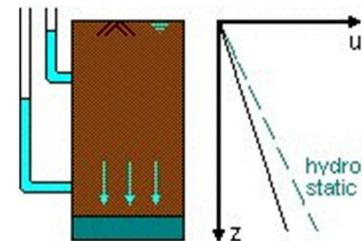
Steady upward flow occurs as a result of artesian pressure when a less permeable layer is underlain by a permeable layer which is connected through the ground to a water source providing pressures higher than local hydrostatic pressures.
