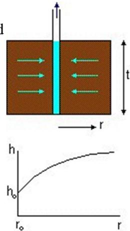
where  $r_0$  is the radius of the borehole and  $h_0$  the constant head in the borehole.
