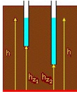
In each diagram there are two points, a small distance  $\Delta s$  apart,  $h_{z1}$  and  $h_{z2}$  above datum.
