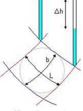
There is an advantage in displaying or sketching flownets in the form of curvilinear 'squares' so that a circle can be insrcibed within each four-sided figure bounded by two equipotentials and two flow lines. Then b = L and  $q = k\Delta h$
