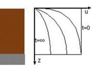
The time-dependent transient change in pore pressure that occurs as a result of some perturbation, and associated change in effective stress is called **consolidation**.
