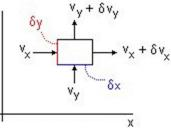
For a rectangular element with dimensions  $\delta_x$ ,  $\delta_y$  and unit thickness, in the x direction the velocity of flow into the element is
