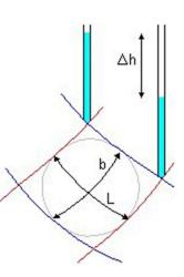
that the seepage force is  $J = i \gamma_w b L$  equivalent to a seepage pressure (force per unit volume) in the direction of flow  $j = i \gamma_W$
