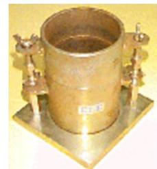
The variation in compaction with water content and compactive effort is first established in the laboratory. Target values are then specified for the dry density and/or air-voids content to be achieved on site.
