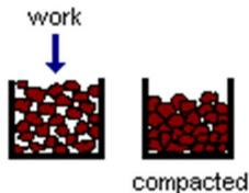
Compaction is a process that brings about an **increase in soil density or unit weight**, accompanied by a **decrease in air volume**. There is usually **no change in water content**. The degree of compaction is measured by dry unit weight and depends on the water content and compactive effort (weight of hammer, number of impacts, weight of roller, number of passes). For a given compactive effort, the maximum dry unit weight occurs at an **optimum water content**.
