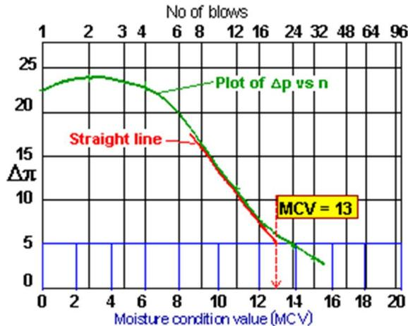
After plotting  $\Delta p$  against the number of blows  $n$ , a line is drawn through the steepest part.
