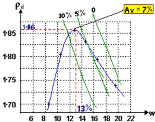
The **optimum air-voids content** is the value corresponding to the maximum dry density (1.86 Mg/m<sup>3</sup>) and optimum water content (12.9%).
