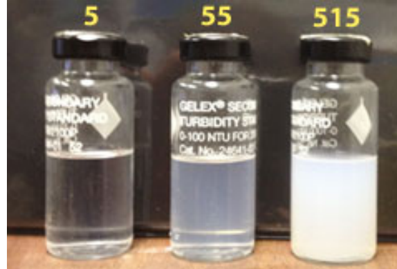
FIGURE 5-2 TURBIDITY IN NEPHELOMETRIC TURBIDITY UNITS (NTU) (USGS, 2014)
