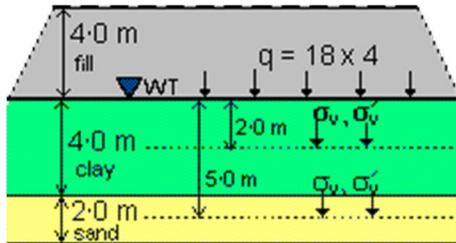
After many years, the excess pore pressures in the clay will have dissipated. The pore pressures will now be the same as they were initially.
