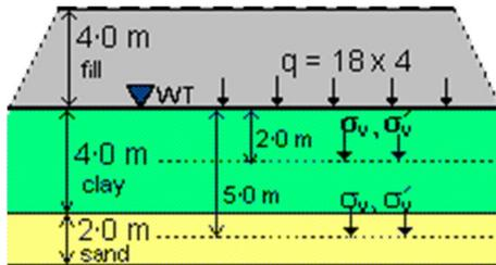
The figure shows how an extensive layer of fill will be placed on a certain site.
