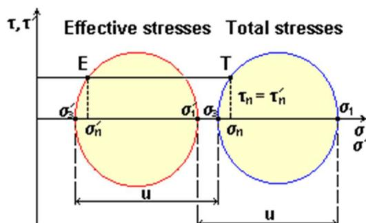
Mohr circles can be drawn for both total and effective stress. The points E and T represent the total and effective stresses on the same plane. The two circles are displaced along the normal stress axis by the amount of pore pressure ( $\sigma_n = \sigma_n' + u$ ), and their diameters are the same. The total and effective shear stresses are equal ( $\tau' = \tau$ ).
