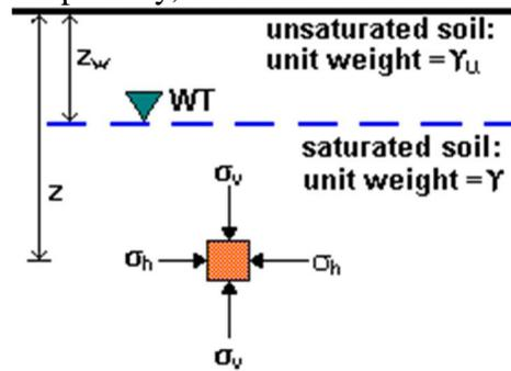
The height above the water table up to which the soil will remain saturated depends on the grain size.
