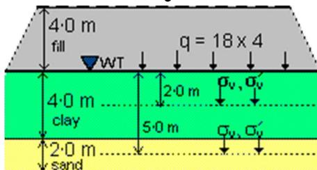
The construction of the embankment applies a surface surcharge:
