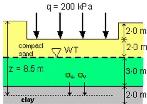
From an initial state, the stresses under a foundation are first changed by excavation, i.e. vertical stresses are reduced. After construction the foundation loading increases stresses. Other changes could result if the water table level changed.
