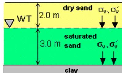
**(a) At the top of saturated sand ( $z = 2.0 \text{ m}$ )**
