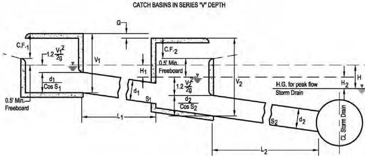
Select a connector pipe size for each storm inlet, and determine the related head loss ( $H_1$ ,  $H_2$ ) by means of a culvert equation, or by Plate 22.3 D-9. The sum of head losses in the series should not exceed the available head, i.e.,
