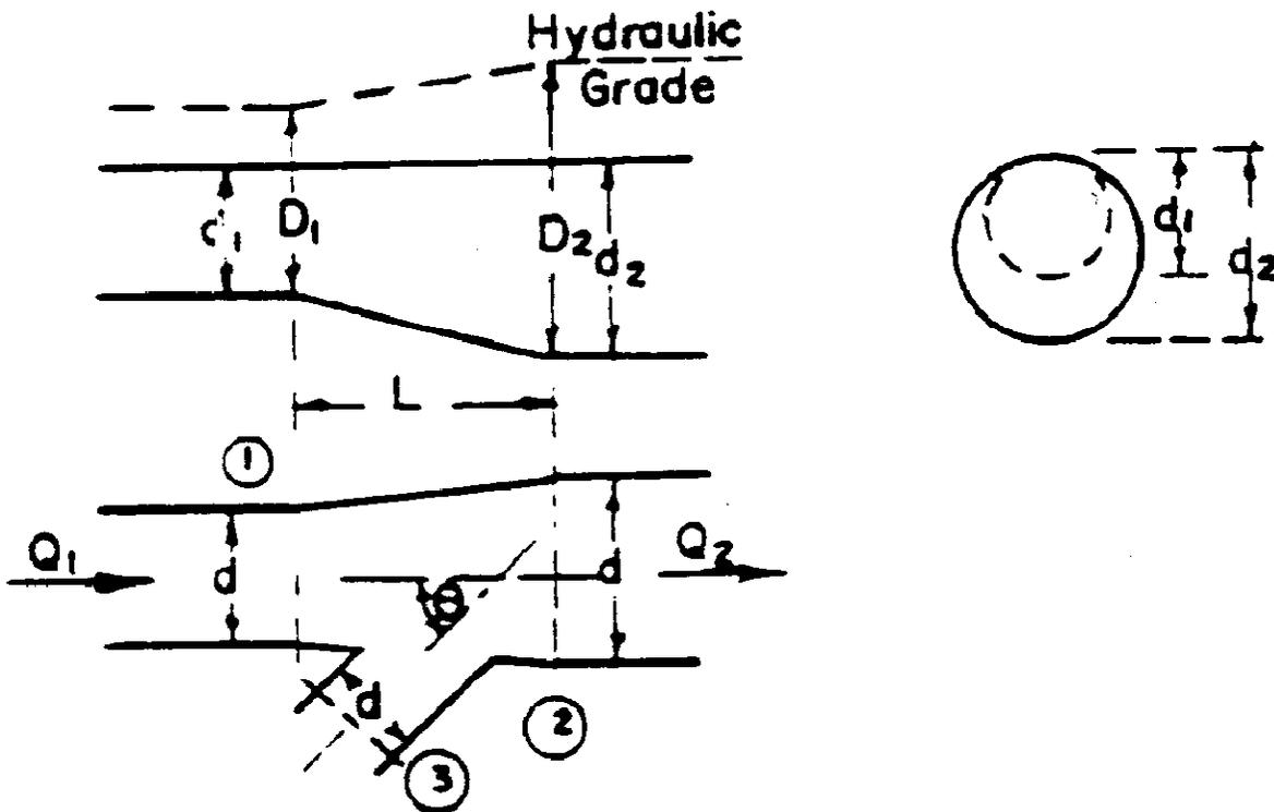
**CASE 5. CIRCULAR CONDUIT FLOWING PARTIALLY FULL, PIPE INLET**
