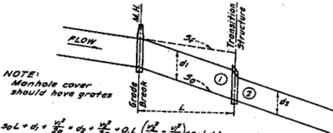
$$s_0 L + d_1 + \frac{v_1^2}{2g} = d_2 + \frac{v_2^2}{2g} + 0.1 \left( \frac{v_2^2}{2g} - \frac{v_1^2}{2g} \right) + s_f L + h_m, \text{ and}$$
