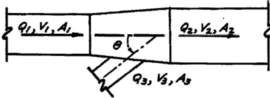
$$\Delta y \cdot A_{avg.} = \frac{Q_2 V_2 - Q_1 V_1 - Q_3 V_3 \cos \theta}{g}$$
