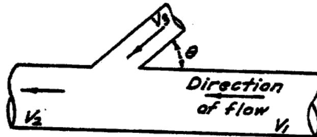
$$h_j = \frac{V_2^2}{2g} - \frac{V_1^2}{2g} - \frac{2A_2}{A_2} \cdot \frac{V_3^2}{2g} \cdot \cos \theta$$
