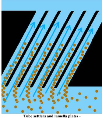
Water flows up through slanted tubes or along slanted plates. Floc settles out in the tubes or plates and drifts back down into the lower portions of the sedimentation basin. Clarified water passes through the tubes or between the plates and then flows out of the basin.
