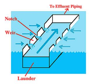
The primary component of the effluent structure is the **effluent launder**, a trough which collects the water flowing out of the sedimentation basin and directs it to the effluent piping. The sides of a launder typically have weirs attached. **Weirs** are walls preventing water from flowing uncontrolled into the launder. The weirs serve to skim the water evenly off the tank.
