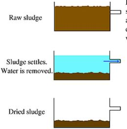
**Lagoons**, which are small-volume storage ponds, are the simplest device used to thicken sludge. These lagoons are filled with sludge and the solids are allowed to settled due to gravity to the bottom of the lagoon while the clear water is pumped off the top.
