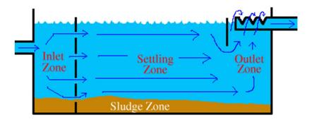
In a clarifier, water typically enters the basin from the center rather than from one end and flows out to outlets located around the edges of the basin. But the four zones can still be found within the clarifier:
