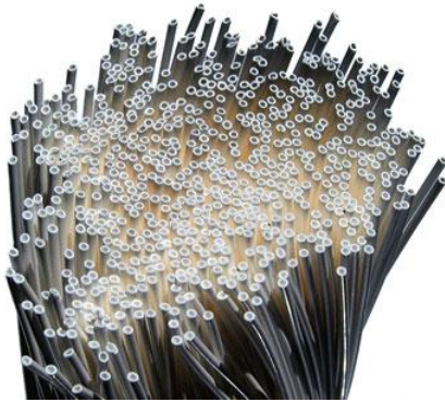
Figure 15 - A Bundle of Fiber Membranes
